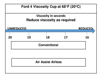
Note: Spraying viscosity and thinning will depend on ambient conditions, spray equipment used, and the desired surface finish.
