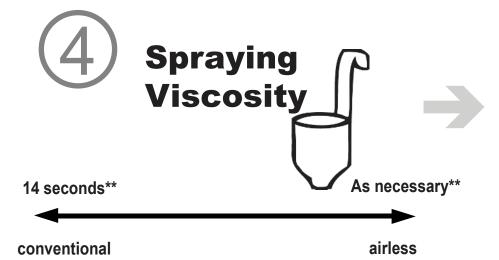
Viscosity: 14 seconds/as necessary using a Ford 4 Cup (white)
