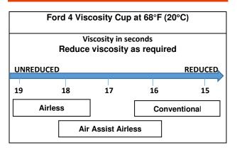
Note: Spraying viscosity and thinning will depend on ambient conditions, spray equipment used, and the desired surface finish.
