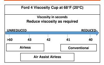
Note: Spraying viscosity and thinning will depend on ambient conditions, spray equipment used, and the desired surface finish.
