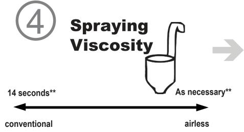
Viscosity: 14 seconds/as necessary using a Ford 4 Cup (white)
