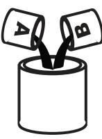
4 Parts Component A1 Part Component B
